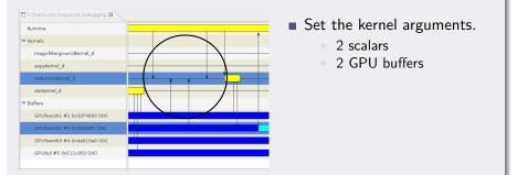
clSetKernelArg(kernel, i++, sizeof(\*ndat),(void\*)ndat); clSetKernelArg(kernel, i++, sizeof(\*in), (void\*)in); clSetKernelArg(kernel, i++, sizeof(\*out), (void\*)out); clSetKernelArg(kernel, i++, sizeof(\*sz), (void\*)sz);
